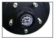
Install hub nose O-ring & adjust bearings per UFP Assembly Instructions.\*
